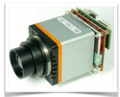
The custom LVDS adapter to the XTM-640 is mounted on the back of the camera. It connects to the E10 LVDS encoder.
