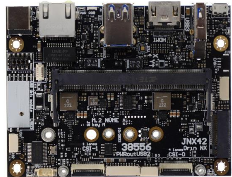
the USB2 connector (J8) is shared with the M.2 key E port
